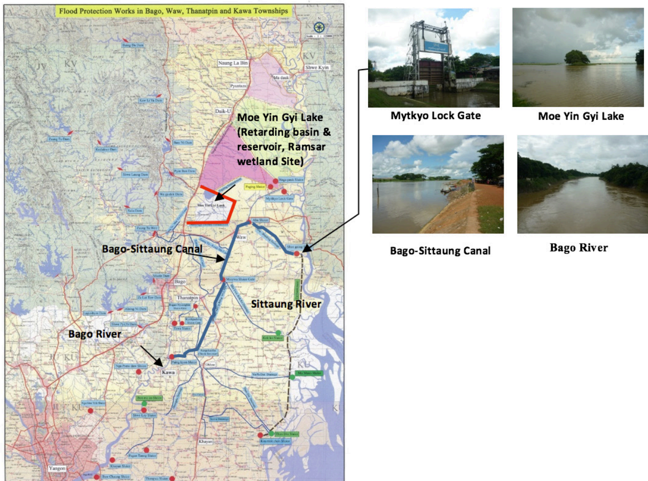
Figure 31. Bago River flood control and navigation canal system (Bago Sittaung Canal) (GP-5.2c)
